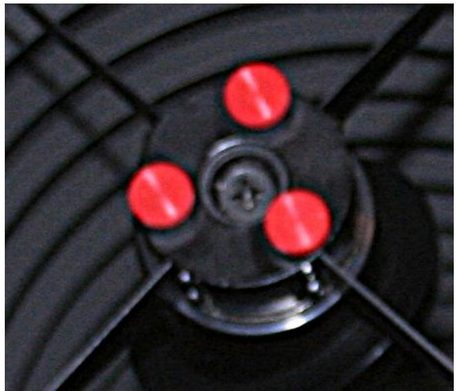
*I had some modifications planned for the the optical tube even as I placed my order for the telescope. Collimating the secondary on the AT8IN requires a screwdriver. Fiddling with a screwdriver in the mouth of your optical tube in the dark, in the field, is a recipe for catastrophe. On receiving the telescope I replaced the screws with M4 screws with press-on knobs from the local fastener store. These work perfectly and I'm not tempting fate when setting collimation.*
