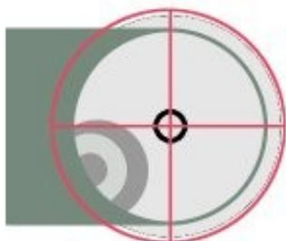
The next step is to put your sight tube back in the focuser and re-adjust the secondary to put the cross-hairs back on the centre spot (things may have shifted when you centred the secondary).
