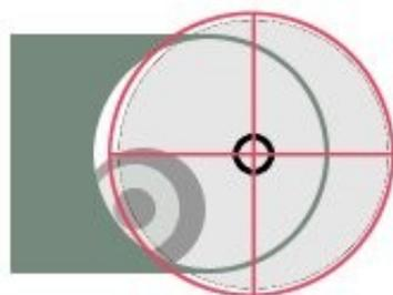
Now place your Cheshire sight tube in the focuser (red). If you are using a 2" to 1.25" adaptor then orient the adaptor so that its tensioning thumbscrew is opposite the one that is holding it in the focuser. Look into the tube and adjust the three (or four) collimating screws on the secondary so as to put the cross-hairs on the primary mirror's centre spot. The grey circle is the shadow of the secondary and Cheshire.
