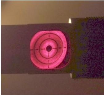
Now put your laser into your barlow and place it into the focuser and turn it on. You'll see the shadow of the primary mirror's centre spot in the cutout of the laser collimator. Adjust the primary cell until the shadow of the centre spot is centred around the hole that the laser is coming out of and then lock the rear cell. You're done. The good thing about this step is that you can do it easily in the field.
