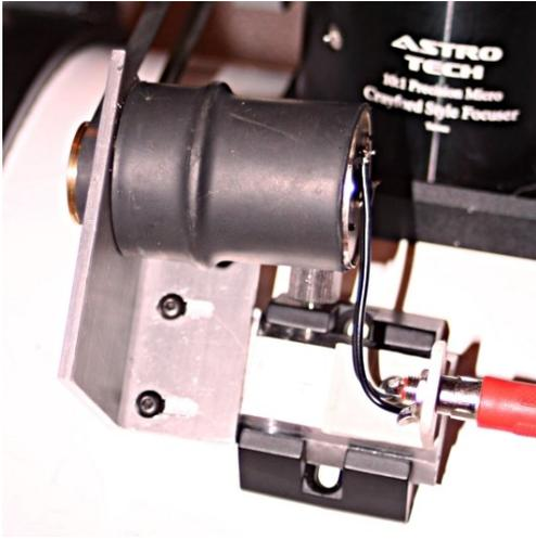
The only 'tricky' part of this came next, the part that would fit into the finder mount. The dovetail used by GSO to mount their finders is a fairly simple 30 degree dovetail. A piece of ½ inch aluminum bar was pulled from the scrap drawer and Dave cut the dovetail angles on a mill using an adjustable-angle vise set to 30 degrees. We left one end of the part square. This would be where the motor bracket would mount. Once shaped everything was squared off and dressed up.
