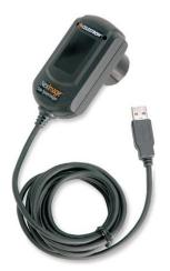
The webcam that I use to guide (when I'm not using my SBIG ST-4) is a Celestron NexImage unit that is, at heart, a ToUCam of some form. This allows me to guide on 9<sup>th</sup> magnitude stars with my 80mm guide scope and down to 10.5 magnitudes with my 8" f/4 newtonian. The drivers are mature and are supplied with the camera.
