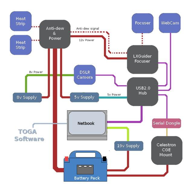
In this schematic the 12v source (whether a battery, my car or an AC/DC supply) is shown as the Canadian Tire Nautilus booster pack that I employ. This has been modified with a set of banana plugs and three decent quality cigarette lighter plugs.
