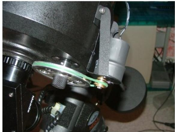
Using a long wire between the motor and the controller can also be useful. This can actually be quite long as voltage drop won't be an issue unless extremely fine wire is used. Enough length means one can be sitting at a laptop several feet from the telescope and still use the powered focuser while analyzing images on the computer screen.
